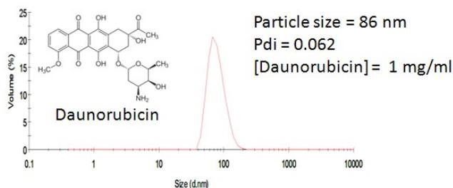
The **Ready-to-load PEGylated HSPC Liposomes with Ammonium Sulfate (Catalog No. PHPC100AS)** includes 10 ml liposomes with 10 mg/ml lipid concentration. The mass ratio of lipids is HSPC: cholesterol: DSPE-PEG2000 = 3:1:1. The concentration of ammonium sulfate encapsulated within the liposomes for drug loading is 200 mM. The buffer is 10 mM histidine,
