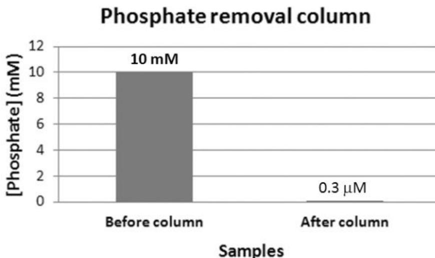
Each Micro Phosphate Removal Column reduces 0.2 ml of 500 mM phosphate to 3 mM. It reduces phosphate from 350 mM phosphate to 0.5 mM; from 175 mM to 0.2 mM and from 10 mM to 0.0003 mM.
